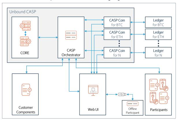
The **CASP Orchestrator** is the heart of the CASP system. It communicates with all parts of the system, initiates creation of the key shares for the vault, manages the different distributed procedures, and acts as the external entry point for the relevant applications, such as the crypto asset applications.
